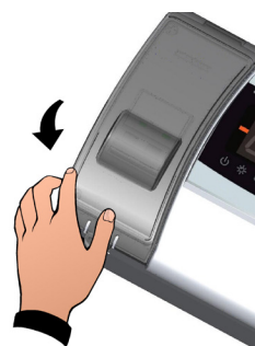
Fig 3. To close the magnetothermal circuit breaker transparent protection.
