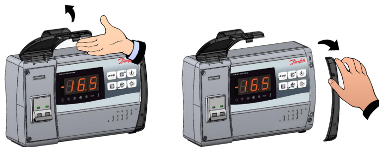
Fig 1. Raise the transparent cover that shields the magneto-thermal cut-out switch and remove the screw cover on the right-hand side.
