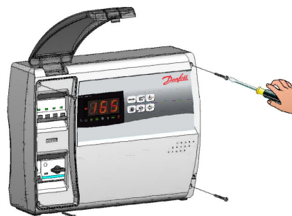
Fig 19. Tighten the front panel using the 4 screws. Refit the cover of the screws on the right side.
