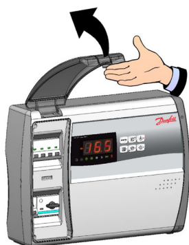
Fig 1. Lift the transparent protection cover of the general magneto-thermal switch.
